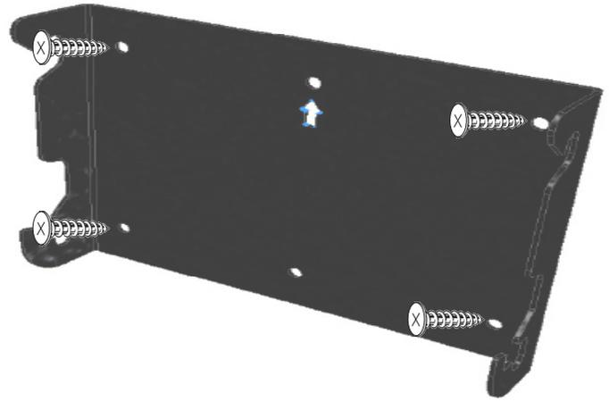
**STEP 1 Secure the portable mounting plate to the mounting surface:** Pre-drill holes using a 1/8" drill bit. Use flat head screws to secure base of bracket to the mounting surface.
