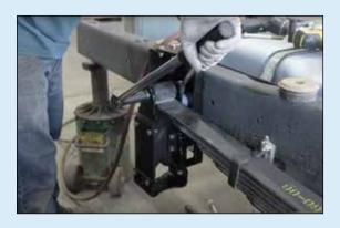
NOTE: The kit may include a jounce bumper plate. If so, install the bolts and tighten and torque to 40 ft-lbs.
