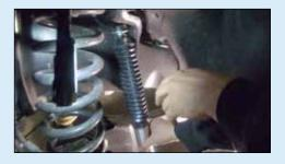
C. Align the bottom mount and install the bottom bolt.
