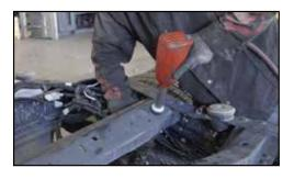
C. Remove the rear OEM shocks.
