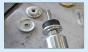
B. Insert the stem through the frame mounting hole.
