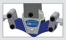
and reinstall the zerk. Make sure the grease exit hole faces the 3 or 9 o'clock posoition for proper grease flow. Reinstall the shackle links and tighten all nuts to 40 ft-lbs. Use a 13/16" wrench to hold the bolt in position while tightening the nuts with an 11/16" or 3/4" socket. If a 3/4" socket is being used to tighten 1/2-20 nuts onto the wet bolts, torque to 80 ft-lbs.
