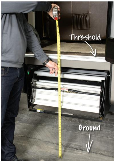
Find your step height by measuring from the top of the threshold to the ground.
