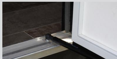
If the door has a strut that prevents it from opening all the way, the step will hit the door. The strut must be removed for proper step installation.
