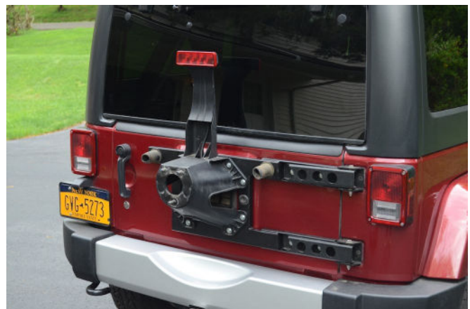
The MORryde Tailgate Reinforcement installed with the factory spare carrier and HD hinges.
