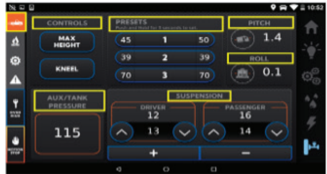
In the above image, "Travel Mode" is indicated by the highlighted (orange) vehicle icon situated at the top left of the Garmin device. Selecting the Travel icon allows the user access to the Air2 suspension travel controls.
